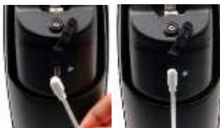
Disconnecting the charger from the prosthesis or mains will be confirmed by a vibration. Reclose the cap properly, since there is a risk of magnetization of metal particles, which would disrupt the connector's connection.
